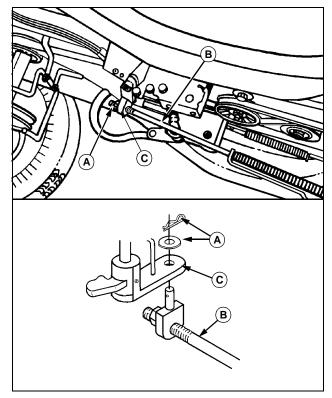
6. Remove spring locking pin and washer (A) holding tension rod (B) to blade drive arm (C).
